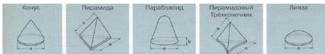
Fig. 2. Forms of abrasive grains on a plastic bond
